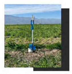
The Arbiter device includes two components; a concentration gradient mast and an augmented soil chamber to track carbon flux, and to monitor soil carbon respiration, and other agronomic indicators.
