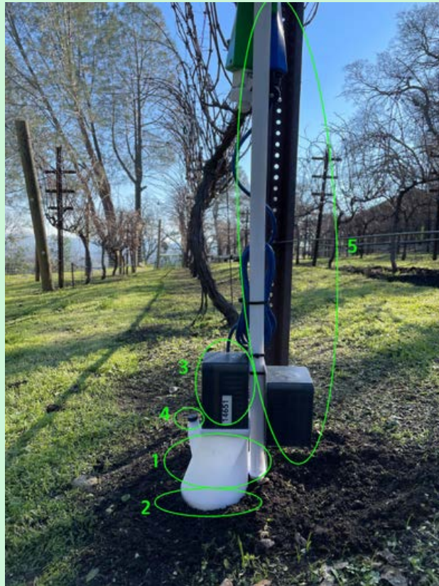
Figure 2: Agrology Arbiter Device, with components identified. 1 - Arbiter Chamber, 2 - Integrated chamber collar, 3 - Sensor Suite, 4 - Proprietary chamber venting system, 5 - Concentration Gradient Mast (not fully pictured)
