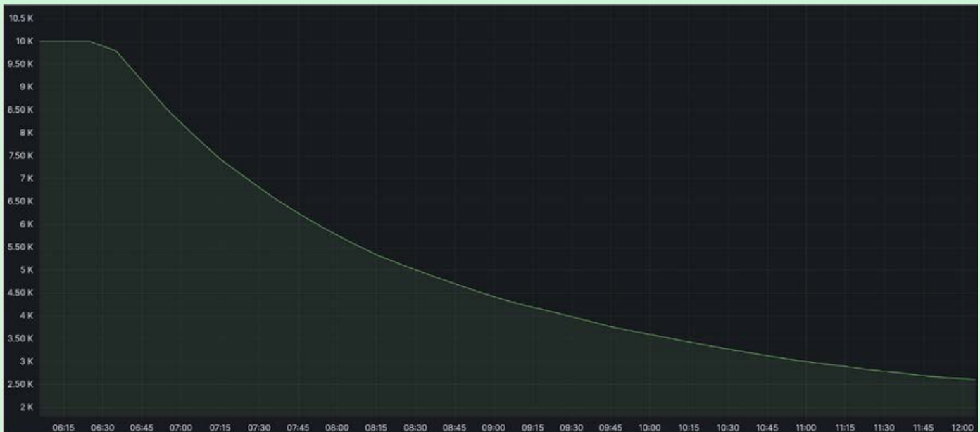
Figure 3: CO 2 Concentration versus time for diffusion factor dK development
